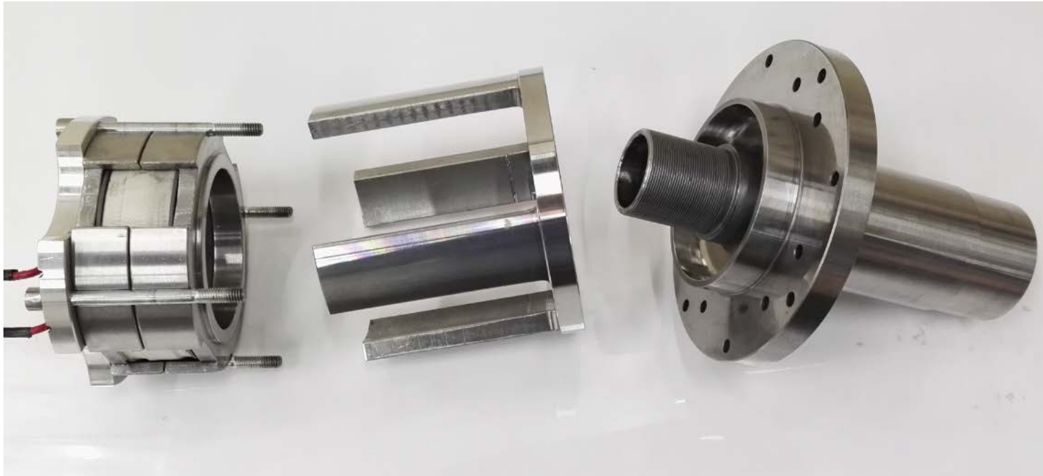
Disassembled engine 'main body' and generator stator
